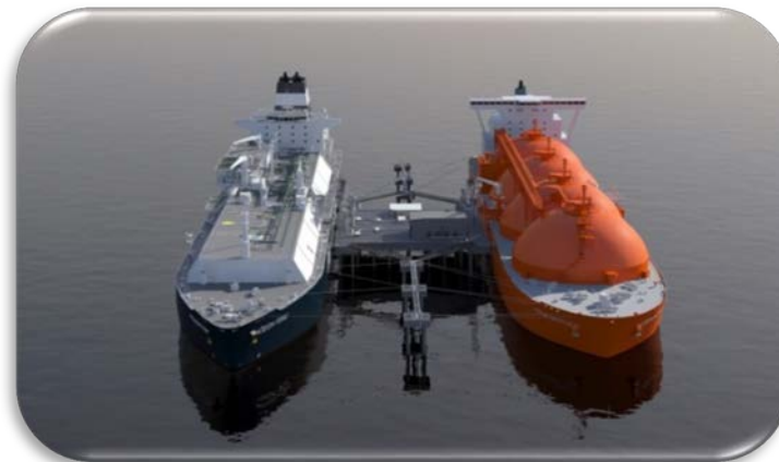
Offshore LNG Terminal using Double-Berth Floating Storage and Re-Gasification Unit Technology (Illustration Photo)
