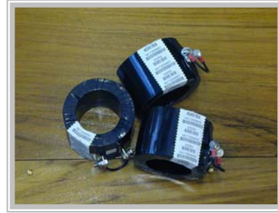
- Tariff metering CTs
