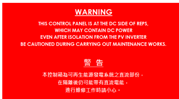
DC Warning Label
