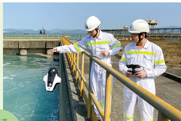
Remotely-operated underwater vehicle is used for inspecting submerged structures
