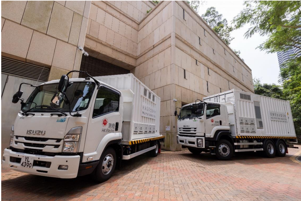
The green mobile electricity supply system, comprising an energy storage truck (right) and a power changeover truck (left), provides uninterrupted temporary relief when normal power is not available.
