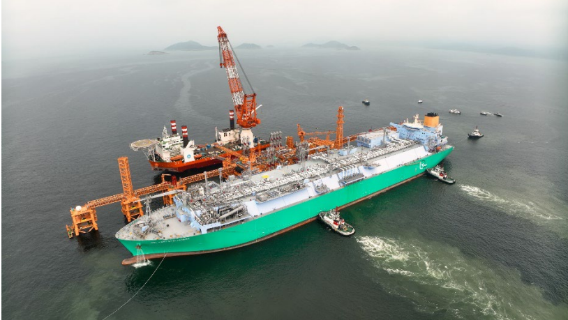
A Floating Storage and Regasification Unit (FSRU) vessel berths at the Hong Kong offshore LNG terminal to prepare for the final commissioning.
